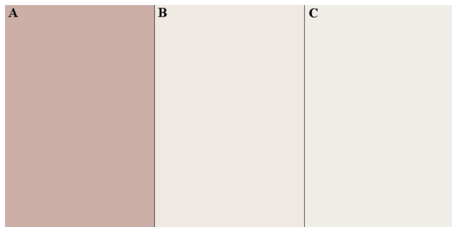
FIGURE 6. Decomposition of the red wine stain: (A) nanosol-treated cotton fabric stained with red wine before exposure to simulated sunlight; (B) sample A after exposure to simulated sunlight for 28 h; (C) control white fabric with no treatment and no stain. The pH of the titania-nanosol solution was 2.
